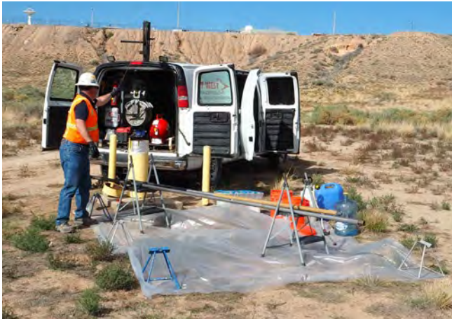
Geophysical logging at groundwater monitoring well TA2-W-19 on the Tijeras Arroyo floodplain.
