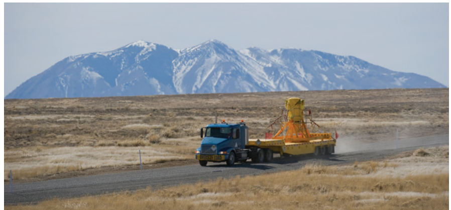
EBR-II fuel was shipped in a Hot Fuel Examination Facility (HFEF)-6 fuel cask on the new haul road between the Critical Infrastructure Test Range Complex and MFC
